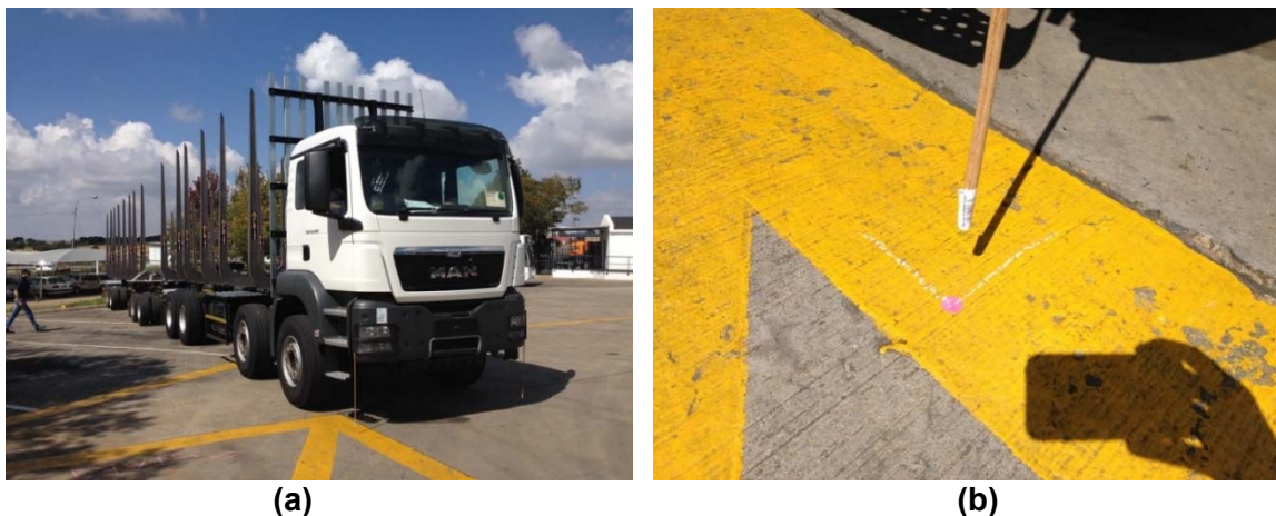
Figure 6: (a) Test vehicle, and (b) trajectory tracking method using dowels and markers
