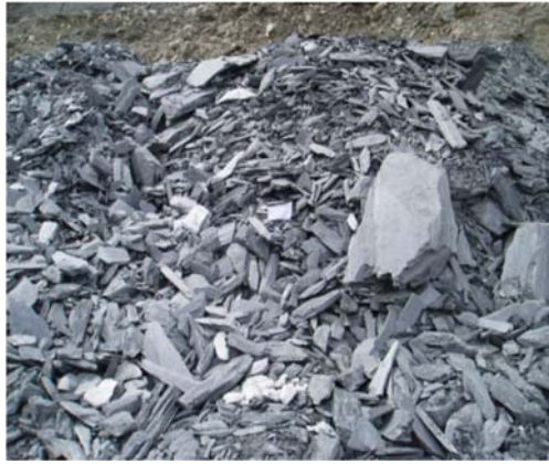
Figure. 2 Weathered phyllite from eastern Ankang of Shitian highway.
