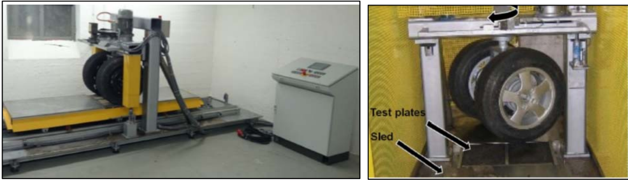
Figure 2 Aachen Polishing Machine (left), detail on the specimens and tire (right) (Wang et al., 2015)
