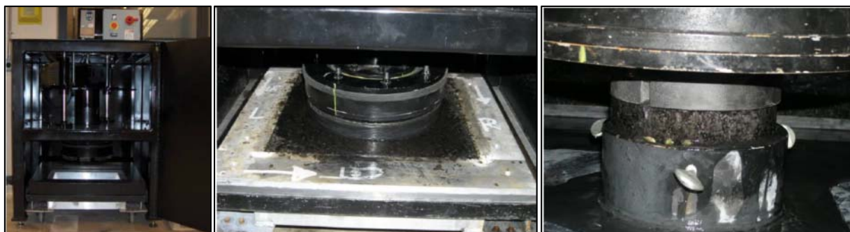
Figure 5 Overall view of Ohio accelerated polishing machine (left), slab specimen mounting (middle), gyrotory compacted specimen mounting (right) (Liang, 2013)
