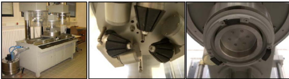
Figure 1 Wehner/Schulze machine (left), polishing unit (middle) and skid measuring unit (right) (BSI, 2014).
