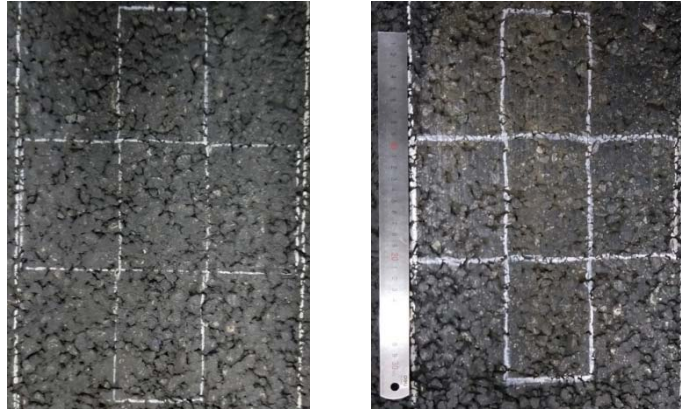
Figure 9 Before abrasion (left), abrasion effect at 19000 load passes (right)
