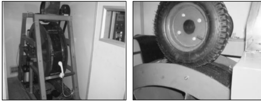
Figure 4 Accelerated Loading System (ALS) (left), detail on tire/specimen interaction (right) (Lei, 2010)
