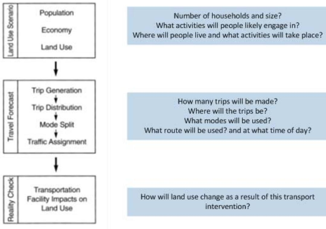
**Figure 2: Adaptation of Beimborn's Overall Forecasting Process**
